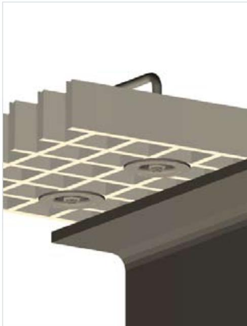
Lifting handles can be supplied in galvanised steel, stainless steel Wst. 1.4301 and stainless steel Wst. 1.4571.
