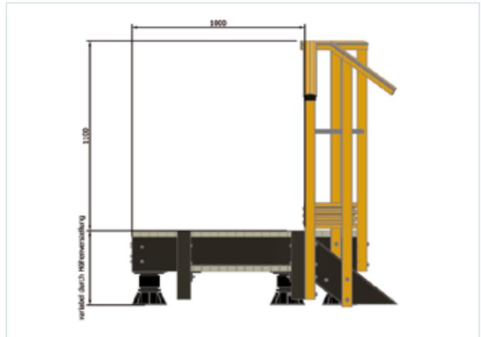
GRP landing composed of GRP profiles as substructure, height-adjustable plastic bases for height compensation as well as a GRP handrail system. These platforms are tailored to the construction requirements of our customers.
