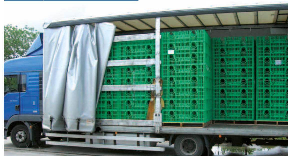
Due care should be taken when loading and unloading, especially at temperatures below 5°C. The Stormbox system elements should be protected against damage and deformation at each stage, from storage, through transport, to the place of installation.
